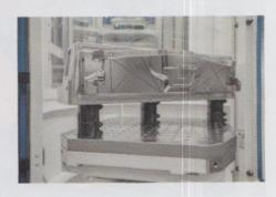
module K10 is positioned at the top, which pulls in and locks the M8 or M10 pull-studs screwed into the workpiece with 10 kN and holds it with 25 kN force.
